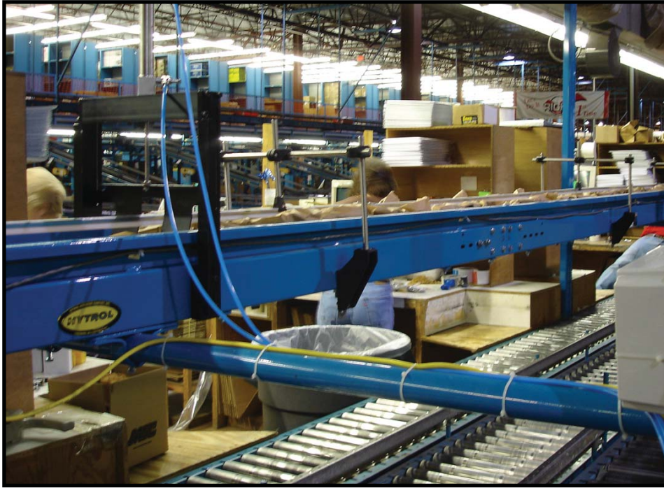
Customized beltway system delivers PadPak packing material to each of the packaging stations on a continuous basis
